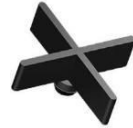
MATRIX Plus shape formed joint strips can be sit in the middle of pedestal and have 3mm thickness. Height 16mm.
